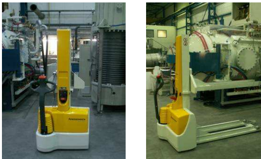
Fig. 26 Electric fork lift loader. 2600lbs (1200kg)
